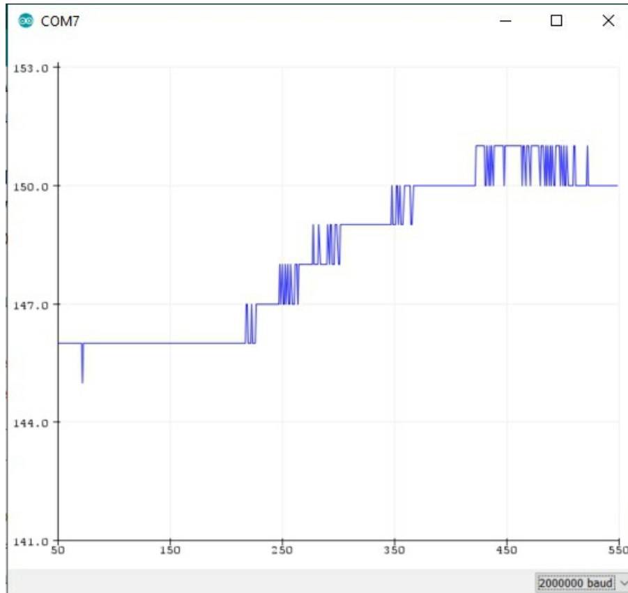
Figure 3.3. A snippet from the temperature sensor ADC reading after touching the sensor. You can see the individual discrete levels of the 10-bit ADC.
